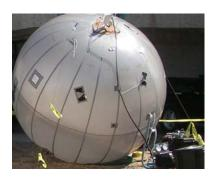
Outside, a representative from GATR Technologies unpacked a satellite balloon from a backpack, and inflated it. Soon thereafter, the balloon was connected via satellite, and was pumping high bandwidth WI-FI to the NIUSR Efforts. Using this creative internet access, members of the NIUSR were able to immediately launch VIA3, a secure collaboration tool, to communicate with remote family, friends, and critical colleagues.
